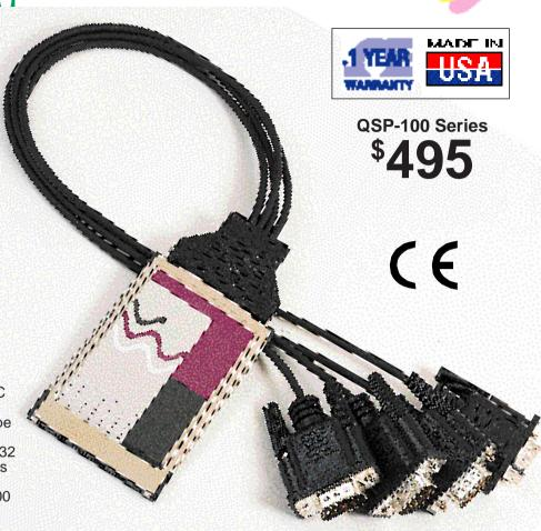
configuration of the QSP-100 upon each card insertion. This will permit the QSP-100 to be "hot-swapped". The QSP-100 will be automatically configured upon each card insertion. A separate enabler program is provided for the configuration of the QSP-100 for those who wish to run the card without card and socket services installed.
